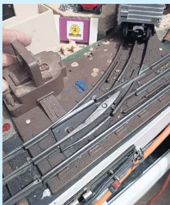
A close-up of the switch shows how a piece of the track is used to divert a train from one section to the other.
